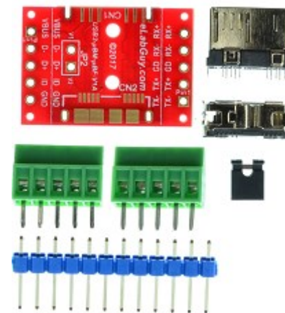
Figure 1: Parts inside the kit (Note: the module is not assembled, user can decide which connector to use on the module.)
